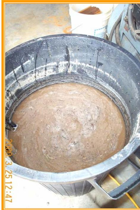
**Figure 1.0 - Construction Water with Glacial Till Silt in Suspension.
