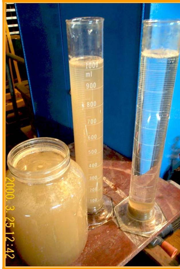
**Figure 6.0 –Glacial Till Silty Construction Water – After 24 hours, no or limited settlement of glacial silt in the 2 gallon jar and 1000 ml column to the left, with clear water and glacial silt in bottom of column, within 5 mins after treatment with the PW Ecell**
