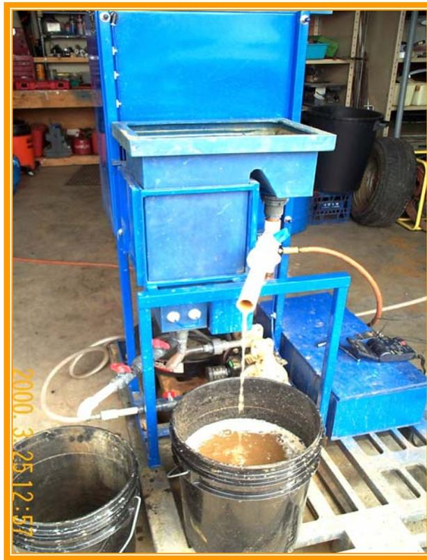
**Figure 2.0 – PW 1.5 gpm Ecell Treating Glacial Till Silt Construction Water**
