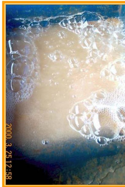
**Figure 4.0 – Construction Water flowing through Alum Plates in PW Ecell - Floc is forming as the Glacial Till water flow over the Chamber Weir to discharge**
