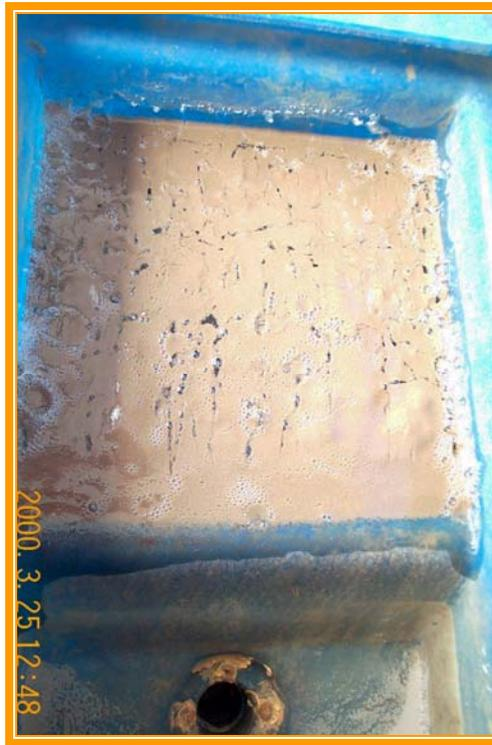
**Figure 5.0 – Glacial Silt on Top of water after treatment with the PW Ecell prior to discharge**
