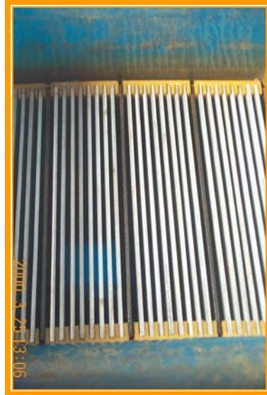
**Figure 3.0 – PW Ecell Chamber with Alum Plates and using steel power plates**
