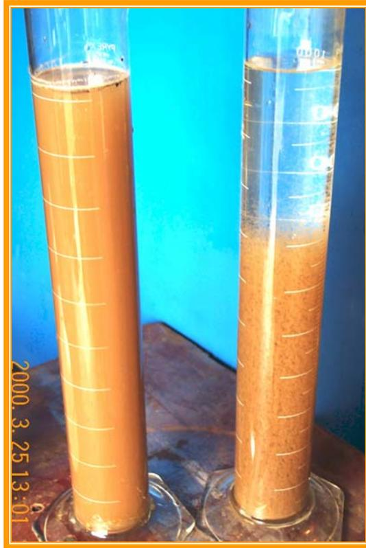
**Fig. 7.0 – Construction Glacial Till Silt water on left and the same water after PW Ecell treatment and after 45 to 60 seconds the amount of precipitation.**
